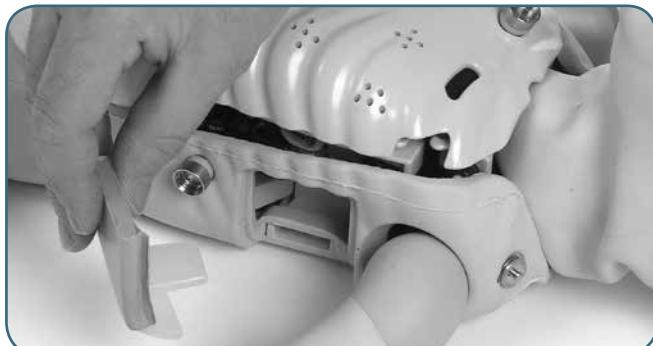
Remove chest tube insertion module from mid-axillary side of simulator.
