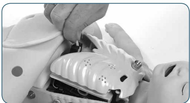
Lift the chest plate assy exposing its underside.
