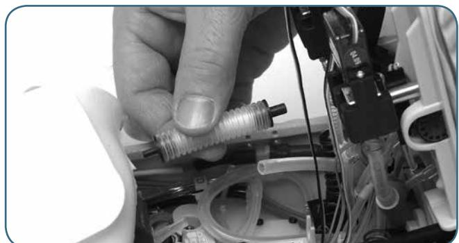
Disconnect the filter assy and replace with a new one.
