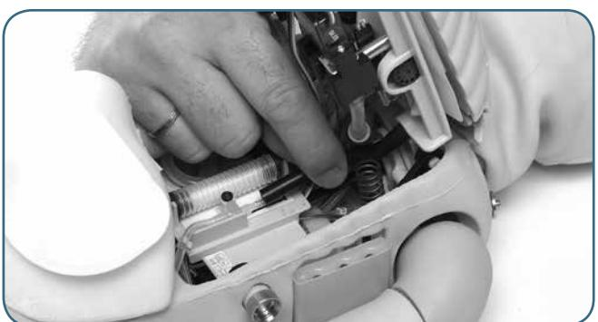
Insert new Pneumothorax Bladder into site cavity and reconnect to the nipple.
