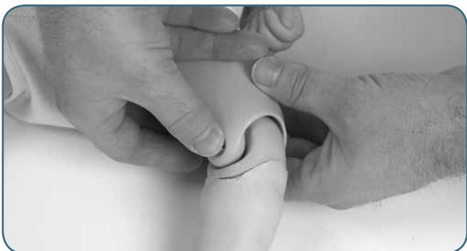
Press the bolt in the knee part out of its seat.
